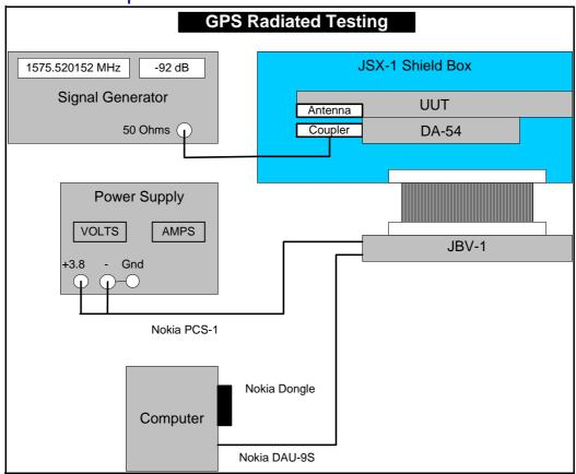
Following is a list of equipment needed for radiated GPS antenna testing:
