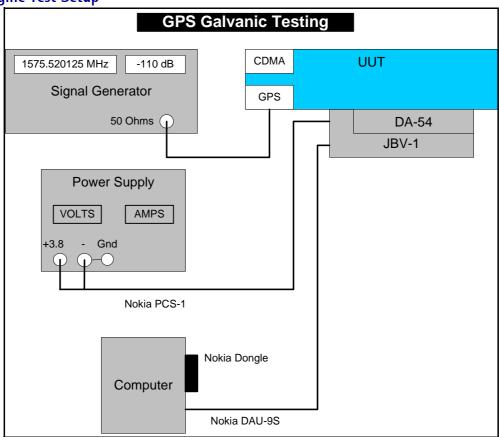
Following is a list of equipment needed for galvanic GPS engine testing:
